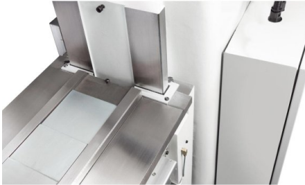
Wide, rigid box ways on Z and Y-axes
