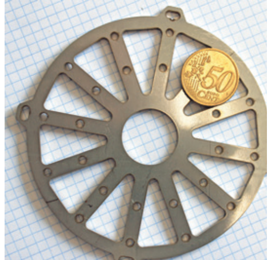
Component cut from a 2 mm thick stainless steel plate using a laser cutter (photo: Klaus Vollrath)
