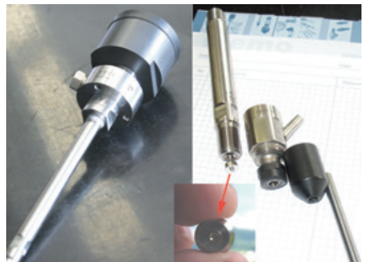
The cutter head of the water-jet cutting system handles pressures up to 4000 bar. In the center of the image: holder with hair-fine nozzle that forms the water-jet (photo: Klaus Vollrath)
