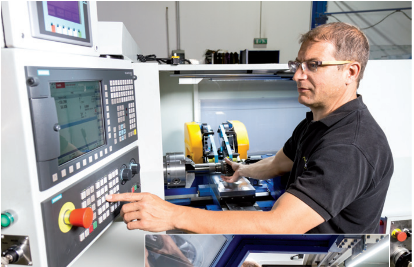
Set up of the CNC lathes' Siemens 828D control with an integrated belt finishing machine
