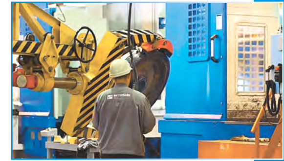
Handling system for loading and unloading
